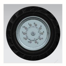
Figure 4-2 Wheel fastening nut tightening sequence
