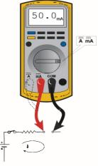
Figure 7-4 Current measurement (direct current)
