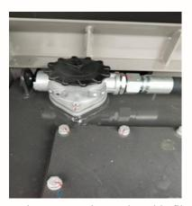
Maintenance point- replaceable filter element.
