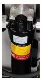
Maintenance point- replaceable filter.
