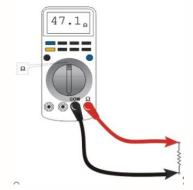
Figure 7-2 Resistance measurement
