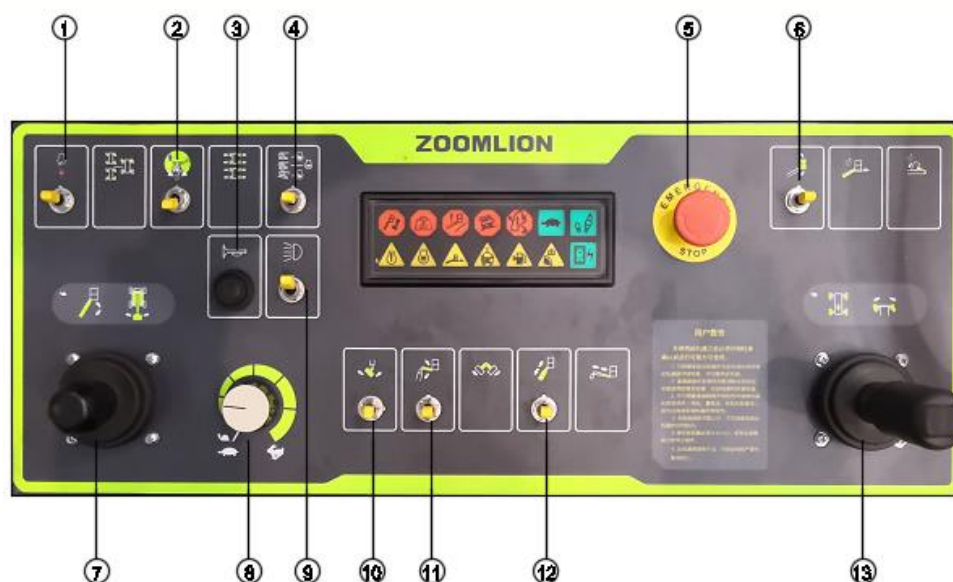
Figure 2-12 Platform Control Panel (The switch number corresponding to the existing function has been identified.)
