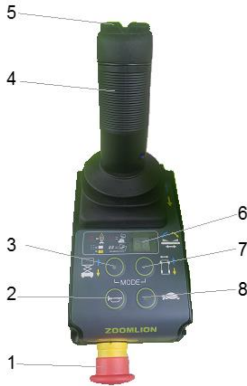
Figure 2-4 Platform control panel
